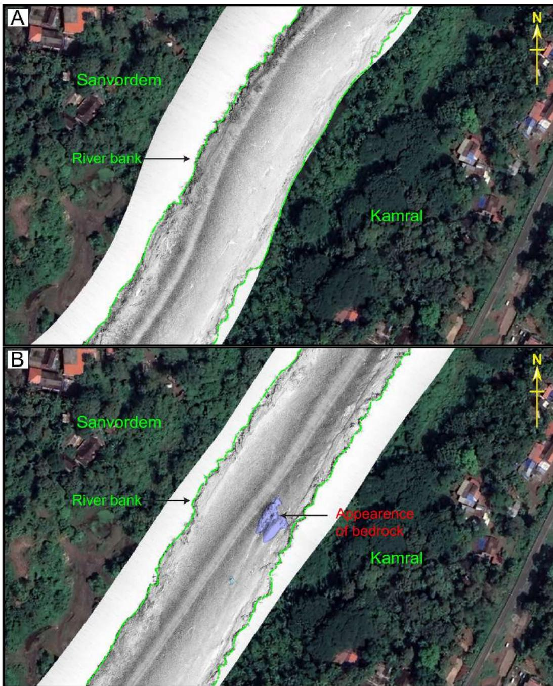
**Figure 28. Side Scan Sonogram acquired near Sanvordem-Kamral (upstream Sanvordem bridge) region during (A) pre-monsoon and (B) post-monsoon seasons. (A) Highlights relatively smooth riverbed morphology. (B) highlights the presence of exposed bedrock indication erosion in this region.**
