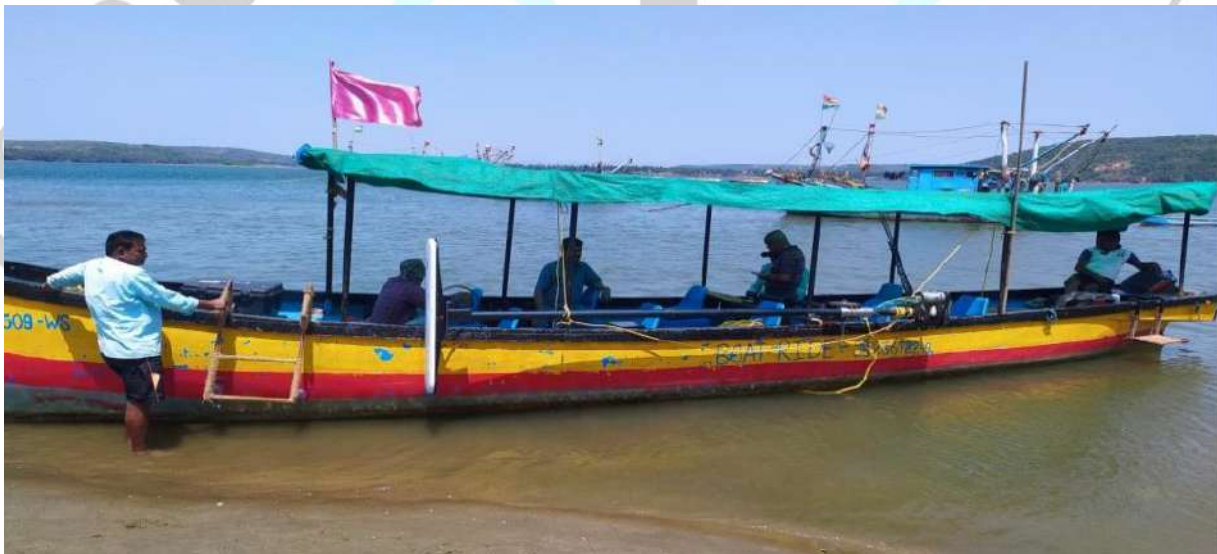
Figure 3. Boat deployed for survey for side scan sonar (SSS) imaging, single beam echosounder profiling, high resolution seismic (HRS squid) survey and geological sampling across the Mandovi river.
